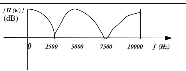
$$\begin{aligned} |H(w)| &= |\cos(\omega T)| & 20 \log |H(w)| &= -3\text{ dB} \\ \arg[H(w)] &= 0, \pi \end{aligned}$$
