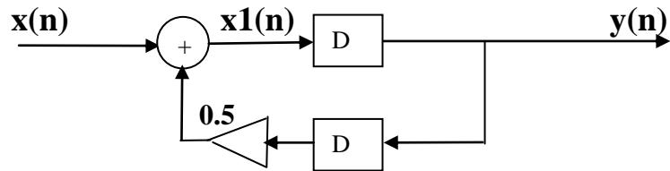
$$\begin{aligned} y(n) &= x(n-1) + 0.5y(n-2) \\ h(n) &= 0.5^k \text{ for } n=2k+1 \\ h(n) &= 0 \text{ for } n=2k \end{aligned}$$
