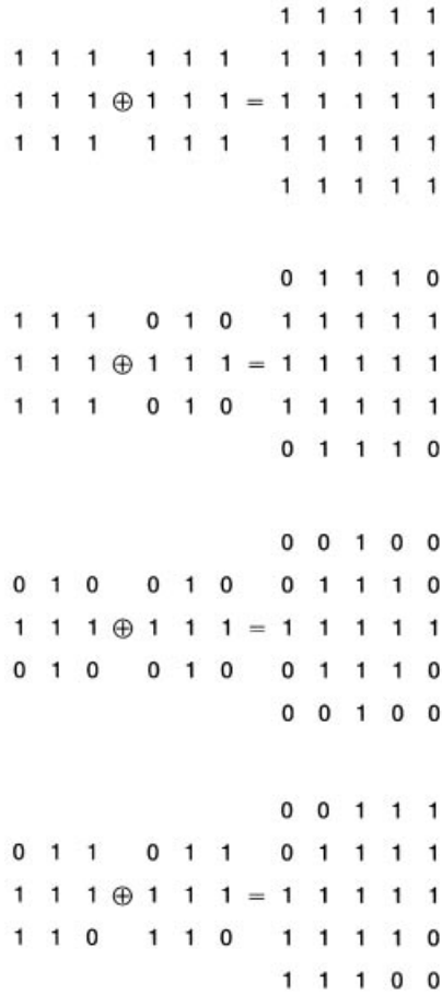
FIGURE 14.4-7. Structuring element decomposition.
