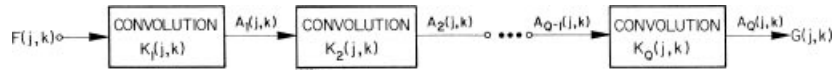
FIGURE 9.5-1. Cascade decomposition of a two-dimensional impulse response array into small generating kernels.
