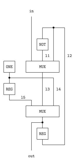
The devices making up this schematic will be modelled with predicates [5]. For example, the predicate ONE is true of a signal out if for all times t the value of out is T.
