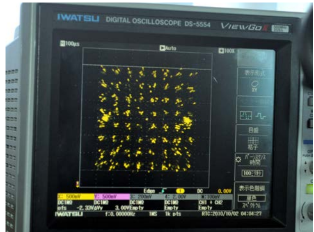
Fig. 19 64QAM constellation at 1000m depth.
