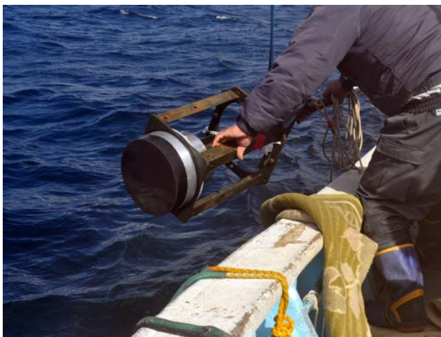
Fig. 18 Rx 4 branches integrated Transducer.
