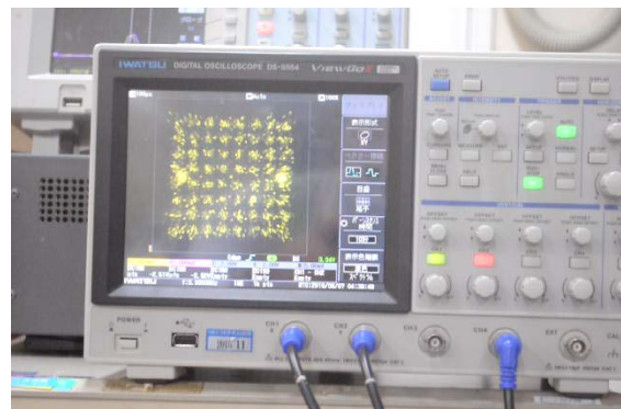
Fig. 12: 64QAM constellation with Doppler Compensation (Receiver moving).
