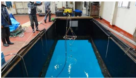
Fig. 10 Ocean Experiment scene at the barge. BS side transducers are submerged in water, and moved up and down vertically with a motor drive. UE side transducers are fixed at bottom of sea.
