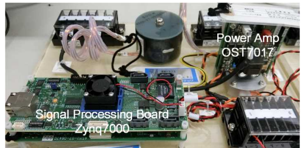
Fig. 8 Developed small hardware system. Zynq7000 ARM-embedded FPGA is used for digital signal processing and OST7010 Power Amplifier drives TX transducer through transformer.
