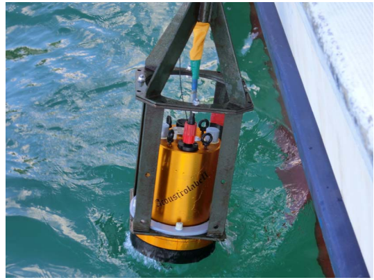
Fig. 10: 8 branches diversity integrated receiver system.
