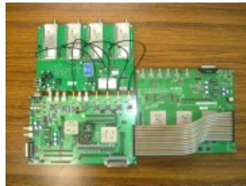
Fig. 6: Implementation Software antenna for ISDB-T reception system.
