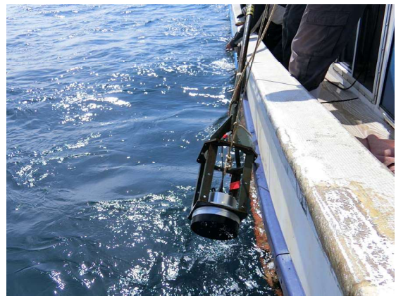
Fig. 10(b): 4 branches integrated receiver transducer. For debugging purpose, Signal processing H/W is separately placed in ship.
