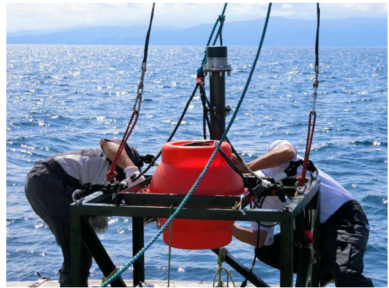
Fig. 10(a): Transmitter system. The top black portion is transducer and red case includes control system and signal processing H/W.
